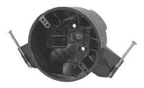
EZ25CN-HW is a 25 cu. in., nail-on, heavy wall ceiling box for new work (construction) applications for residential and light commercial projects. It is a heavy duty new construction (new work) ceiling box to use where a more durable electrical box is preferred. The harder shell is designed to resist flexing and hold its shape. It features enhanced angled nails for easy mounting between studs and 5 heavy-duty wire clamps for EZ and secure wiring.
